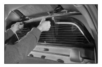
4. With the rear glass tilted toward you, lift it out from the lower window frame channel. Use the grab handles to assist you in removing the rear glass.
